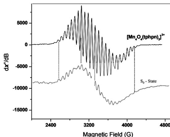
Figure. EPR spectra of  $[(Mn_2O_2)_2(tphpn)_2]^{3+}$  (top) and Photosystem II  $S_0$  state (bottom).
